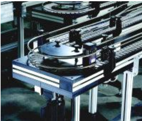
System SBF-2000 Curve Segment
