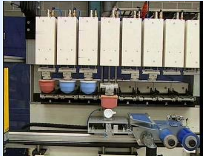
Modular pad printing system up to 8 colors; with Pad Cleaning Device
