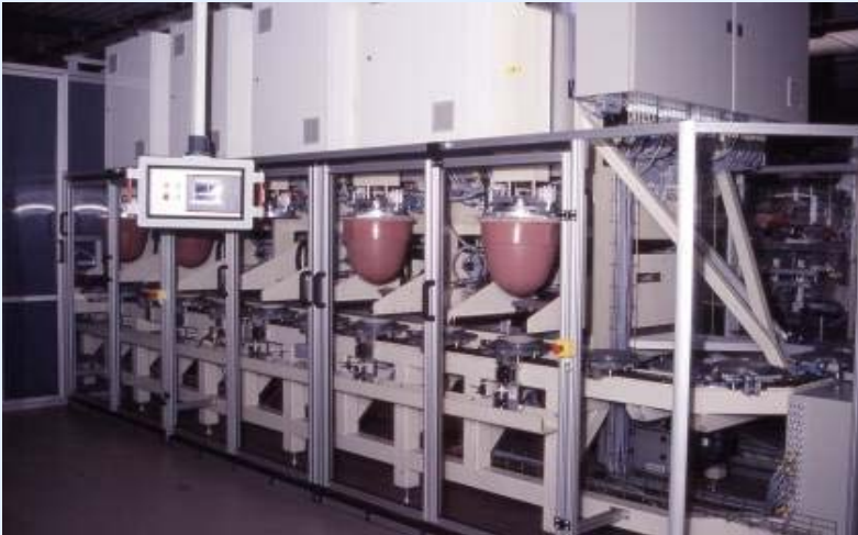
12 color pad printing system to print on ceramic plates
